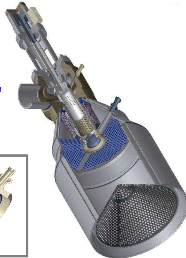
Figure 5: Isometric view of a steam conditioning valve
